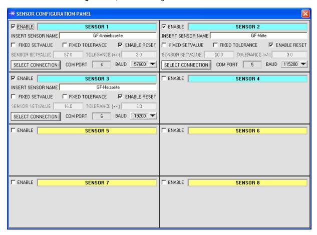
If data should be recorded from a sensor, the sensor must be activated with "ENABLE".
