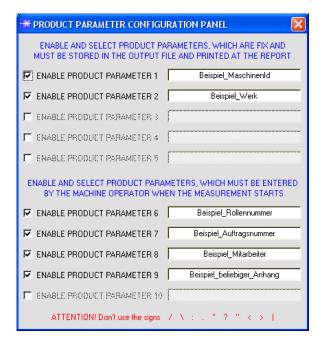
There are 5 parameters that can be individually entered. All these data are fixed and are, if they are enabled, saved in the file and printed in the report. Parameters 6 to 10, if they are enabled, must be entered by the operator after pressing "Start". These data also are saved in the file and printed.
